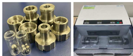
Fig. 1. Pictures of stainless balls and reaction jars (left) and a mixer mill MM200 (right)..
