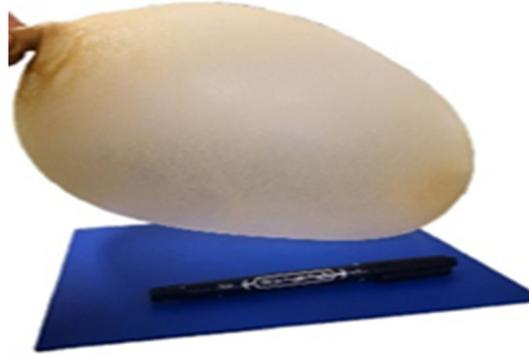
Fig. 3 Inflatability of wood powder-PVA-HPMC-borax hydrogel (Sample 5 in Table 1).
