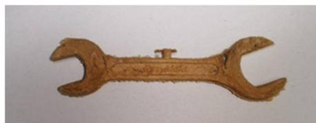
Fig. 2 Inject molding prototypes made from kneaded material with wood powder, HPMC and water.
