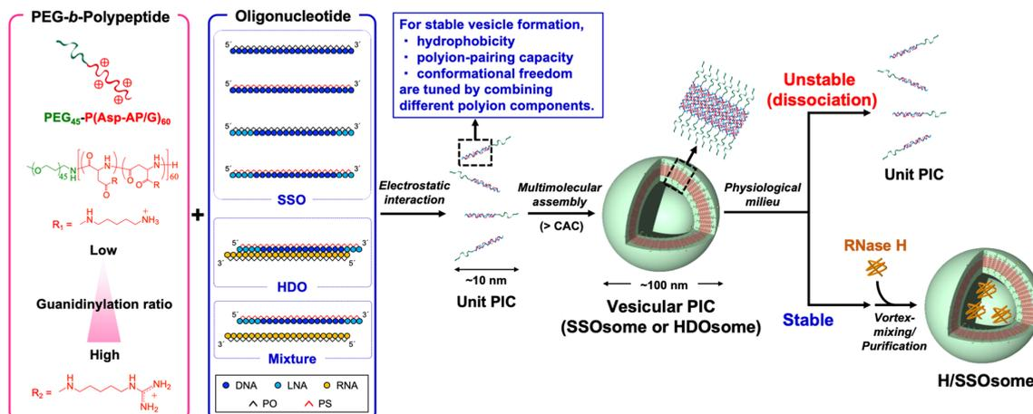
[Schematic Illustration Depicting the Fabrication of Noncovalently Stabilized Vesicular PICs Using Cationic PEG-b-polypeptides and Anionic Oligonucleotides]
