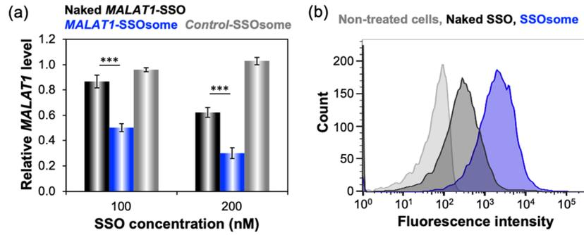
Biological activities of SSOsomes. (a) Gene knockdown efficiency determined by qRT-PCR. The cells were incubated with naked MALAT1-SSO or MALAT1/Control-SSOsomes for 48 h. (b) Cellular uptake efficiency determined by flow cytometry. The cells were incubated with free AF647-SSO or AF647-SSOsome at 200 nM SSO for 4 h.
