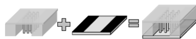
Fig.1 Schematic illustration of the a three-dimensional dielectrophoresis device equipped with a micro-fluidic channel with built-in pillar arrays.
