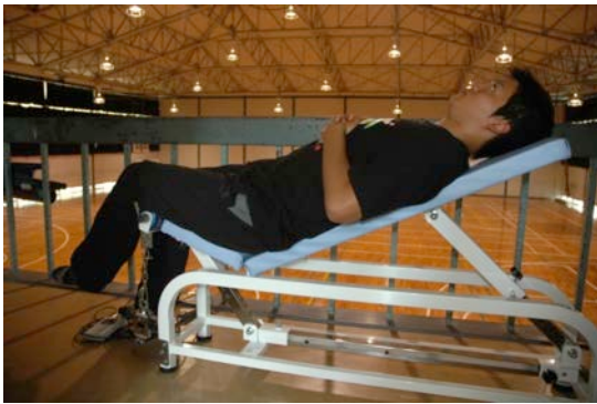
図3 傾斜座位型股関節筋力計
