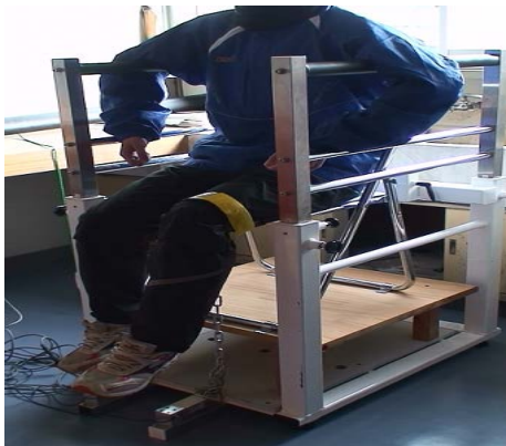
図1 座位型股関節筋力計
