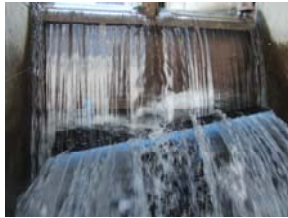
(b) Suppression of nappe oscillation with equipment
