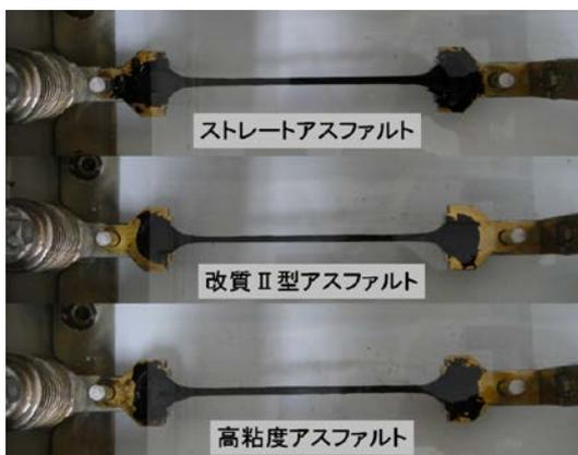
図3 the force ductility test 載荷中の供試体形状 (300mm 変位時)
