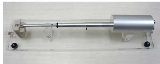
Fig. 1 A manipulator with a load detection function.
