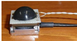
Fig. 2 Hybrid tactile sensor system
