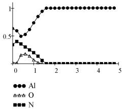
formed at these doses. This is in stark contrast to for example the oxidation of Al, where a protective layer prevents further oxidation. Using the depth profiling technique developed as subject (4)of this project, information on the constituents of the thin film was obtained. The results are shown in figure 4, where it is clear that we can see deep penetration of N into the sample. A similar analysis can be performed for each of the 4 components to the N 1s peak - these
