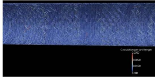
Fig. 2 Vortex element distribution at the half length of the pipe. ( $C=2.0$ , color: vorticity strength)
