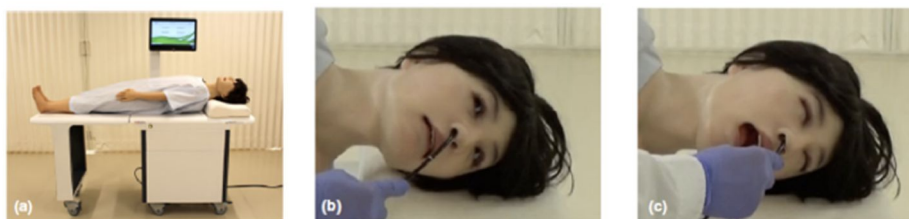
図1. 内視鏡用シミュレータロボット“ミコト” Development of a novel humanoid-robot simulator for endoscope with pharyngeal reflex and real-life responses.
