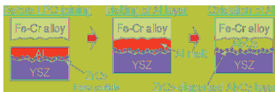
Fig. 1 Procedure of liquid-phase-oxidation (LPO) joining between Fe-Cr alloy and YSZ to disperse \text{ZrO}_2 particles in \text{Al}_2\text{O}_3 layer.
