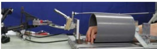
Fig.2 Experimental setup for the Bowden cable control
