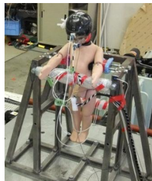
Fig.1 Vibration experiments using a six-month-old-infant dummy
