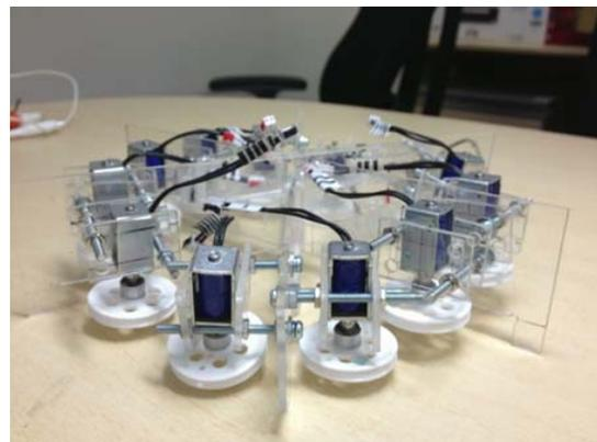
Fig.6 Solenoid valve mechanism.
