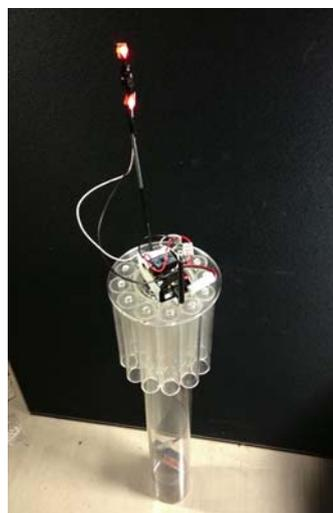
Fig.3 Configuration of the spar-buoy model.
