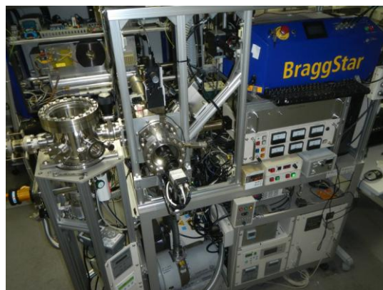
Fig. 1 Pulsed laser deposition system adapted for very wide-gap material deposition.
