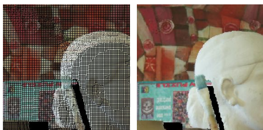
Fig.3: (left) DIBR-synthesized image for virtual viewpoint closer to the 3D scene, (right) interpolated image using our proposed graph-based algorithm
