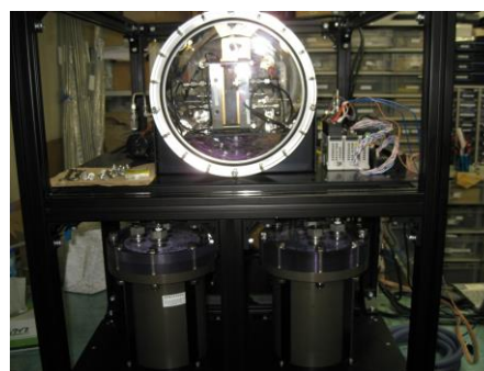
Fig.2 Evaluation System with Pressurization Function
