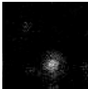
Figure 6. Typical fluorescence image of PTCDI-PNIPAM spin-coated on a cover glass ( 10 \mu\text{m} \times 10 \mu\text{m} ).
