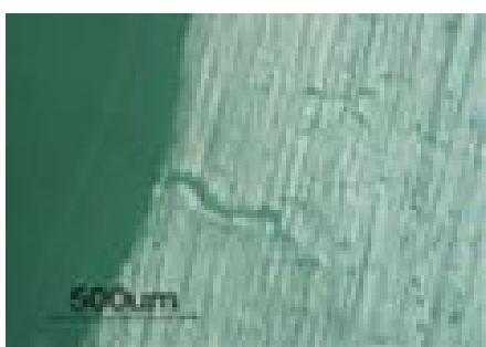
Fig. 6 Crack initiation in pearlite material under fatigue loads (microscopic image with 50 times zoom) in 14 th AE hit.
