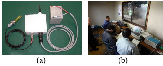
図 5 Piezoelectric vibration sensor for structural health monitoring system
