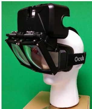
図 1. 光学透過式 HMD の試作例、University of North Carolina at Chapel Hill, "Converting Commodity Head-Mounted Displays for Optical See-Through Augmented Reality", 2015.4 より
