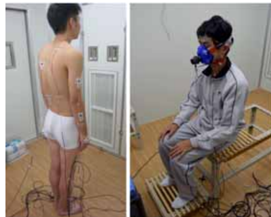
Fig. 1 Nude subject attached sensor of heat flux meter (Left)
