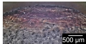
Fig. 5 Surface of \text{SiO}_2 coated tool after grinding
