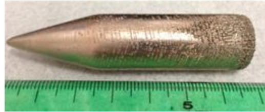
Fig.1 Photograph of \text{Cu}_{75}\text{-Ni}_{20}\text{-Fe}_5 alloy single crystal
