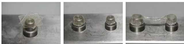
Fig.1 Fiber Net, glass Fiber and fiber-reinforced resin bridge (Design3).
