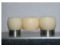
Fig.1 Fiber Net, glass Fiber and fiber-reinforced resin bridge (Design3).
