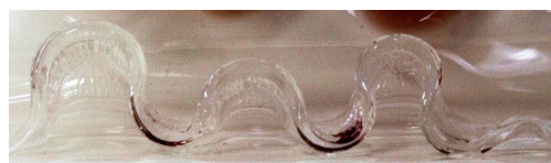
Fig. 6 Top view of the buckling of the bi-layer gel.
