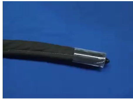
Fig.7 Developed actuator equipped with the head unit
