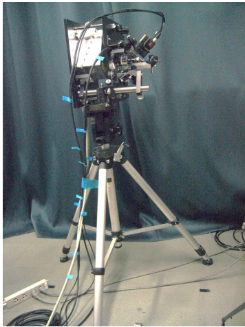
Fig. 2 Bi-directional measurement interferometer constructed on tripod
