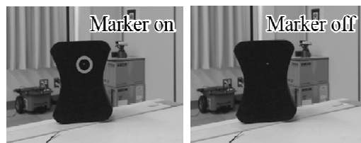
Fig.6 Image example of our proposed laser spot marker
